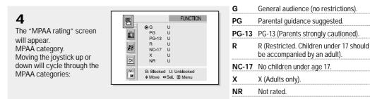
While a particular category is highlighted, move the joystick to the right to activate it. A blinking letter ("U" or "B") will be displayed. Move the joystick up or down to select "U" or "B".
